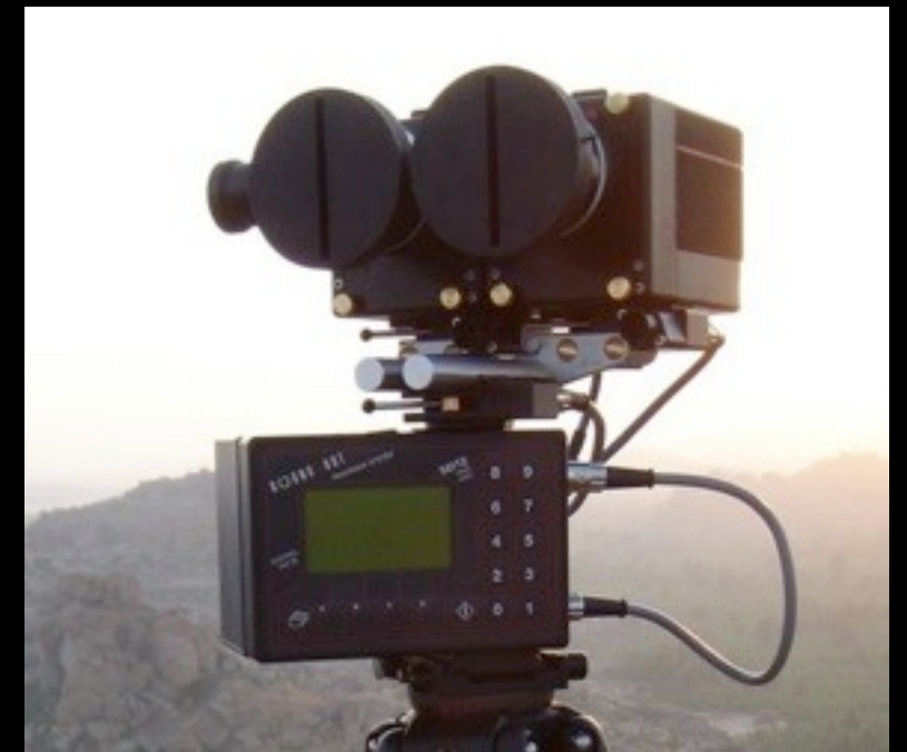
Place-Hampi stereo panoramic still slit camera system (It takes about a minute to complete a rotation.)
