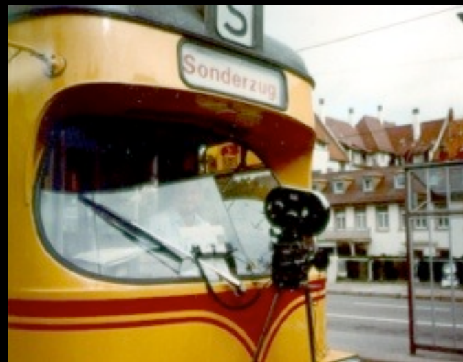
Karlsruhe Moviemap, ZKM, 1990 odometer triggered wide-angle cam
