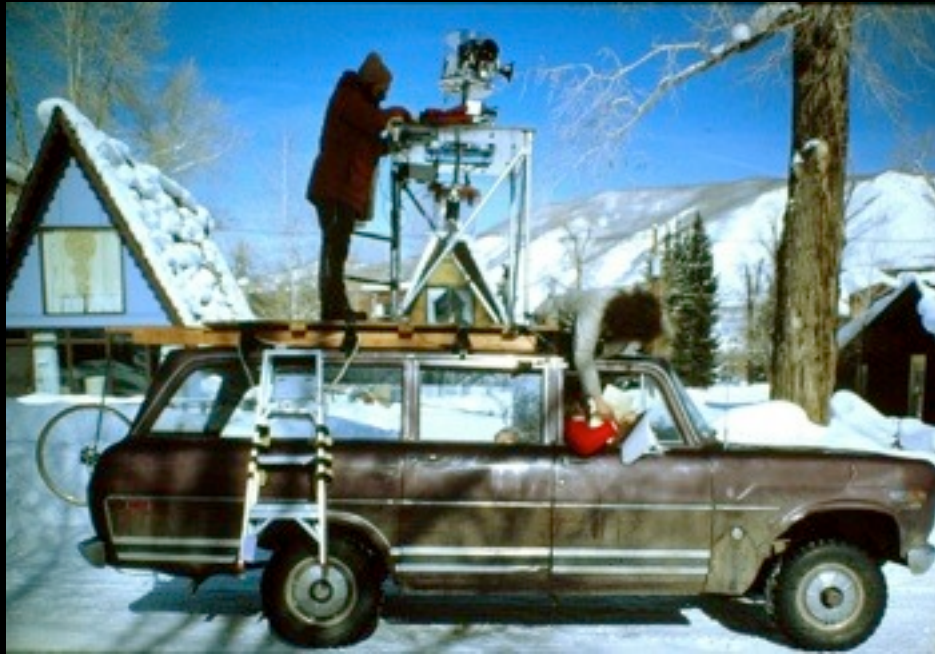
Aspen Moviemap, MIT, 1978 bike wheel triggered pano cams
